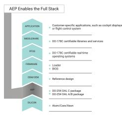
Figure 1. Certifying an avionics system requires addressing multiple levels
