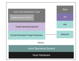
Figure 2. Simics enables deterministic virtualized hardware simulation
