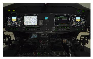
Figure 2. Northrop Grumman's OpenLift™ Modular Open Systems Architecture (MOSA) Cockpit (UH-60V) (Source: Northrop Grumman)
