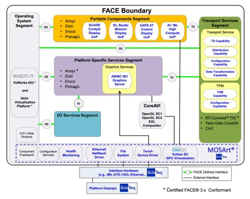
Figure 7. MOSArt alignment with FACE Technical Standard reference architecture (Credit: FACE Reference Architecture, The Open Group)
