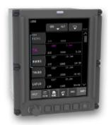
Figure 5. Touchscreen Control Unit (Source: ScioTeq)
