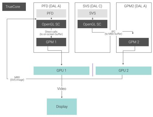
Figure 11. Dual GPU architecture
