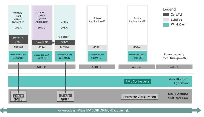
Figure 12. ScioTeq display platform architecture with example configuration
